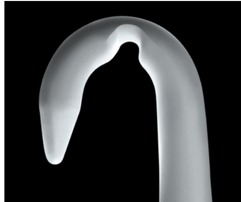
Wear to the inside area of the hook (without chrome-plating)
